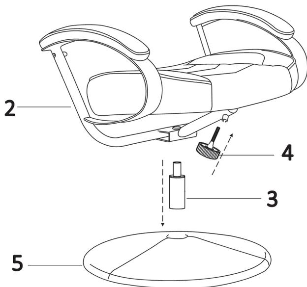
1.1 Install the column **#3** to the base **#5**, the seat **#2** to the column **#3**.
