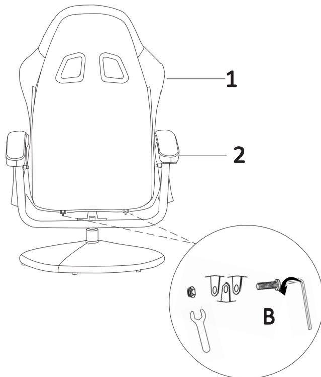
Connect the backrest **#1** and the seat **#2** with the screws **#B**.
