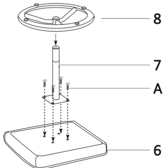
Install the column **#7** to the seat cushion **#6** with screws **#A**.
