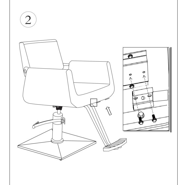
Please note that the foot rest and seat connection screws are pre-installed under the seat.
