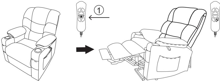
1. press the button ① can recline the footrest continuously.
